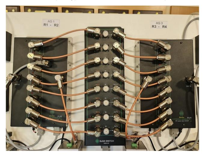
The right hand side of the 8xAB switch is normally closed so the AG connected to the right hand side has the antennas available at start.
