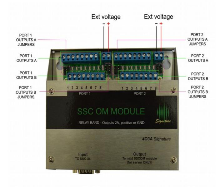
Internal voltage is used for testing and programming, and it is strongly recommended to use proper external power supply and set jumpers to EXT. Internal power supply in SSC XL is 1A, which is on the margin if all relays are in use.
