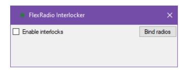
**Bind radios** will display a list of the FlexRadio serials on the network.
