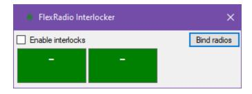
The radios will display as rectangles, the color will show the status of the radio. **Green** for **not active PTT** and **red** for **active PTT**, the interlocker radio as **blue**.
