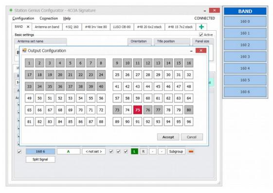
Every row represents an OM. You can daisy chain up to 6 modules for a maximum of 96 outputs. Rows 1 trough 16 represent the first OM. Rows 17 trough 32 represent the first OM and so forth.
